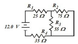
**8.** What is (a) the total resistance of the circuit, (b) the total current in the circuit, (c) the power developed in the circuit?
